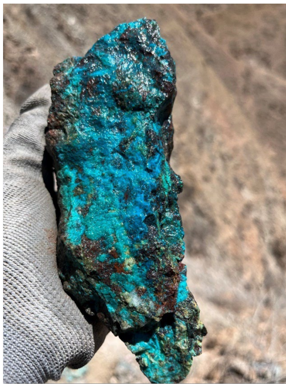
Figure 1: Cinto Project surface grab sample 17142 with visible copper oxides and silicification returned 7.14% Cu (see Appendix 1 for details) 2
