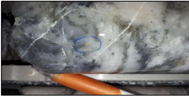
Figure 1a: Visible gold in hole HUD002 at 129.7m
