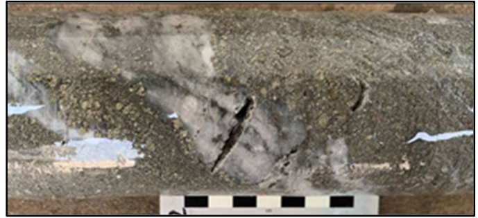
Figure 1b: Strong pyrite-silica alteration HUD002 at 110m
