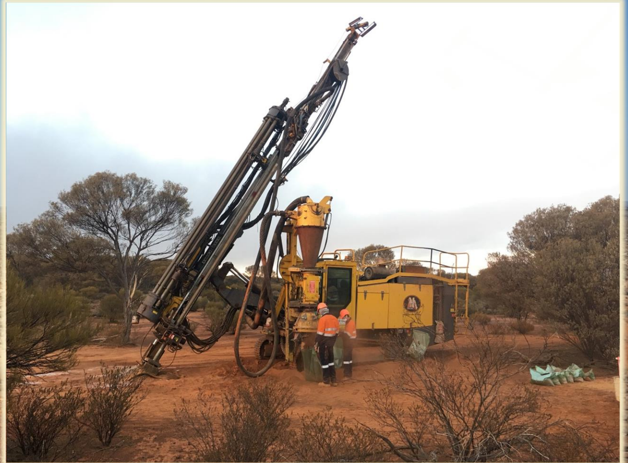
Reverse Circulation drilling at Fenceline Gold - 28 May 2018
