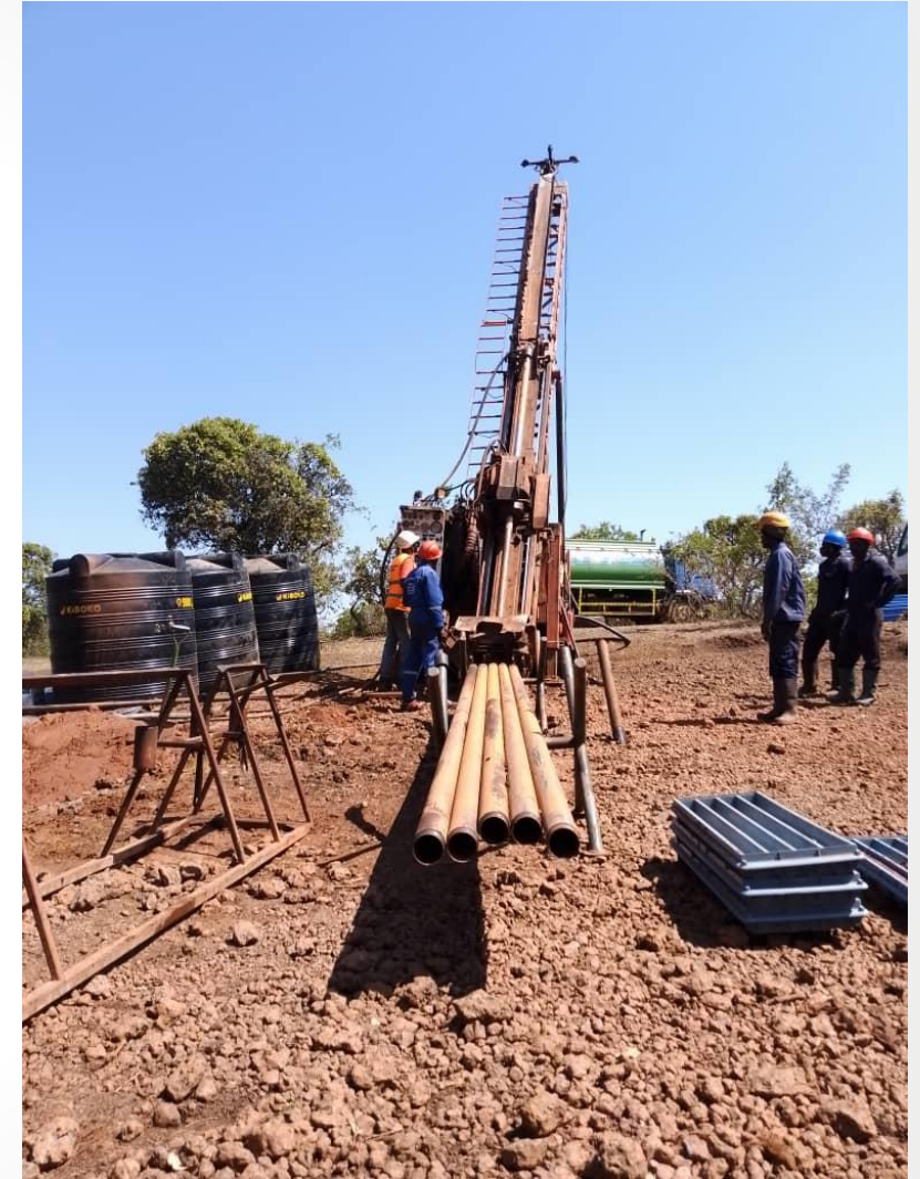
Diamond Drilling at Luhuma Central LUHC003
