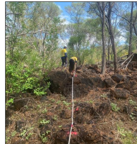
TNC exploration team rock chip sampling gossanous breccia at Alpha Gossan
