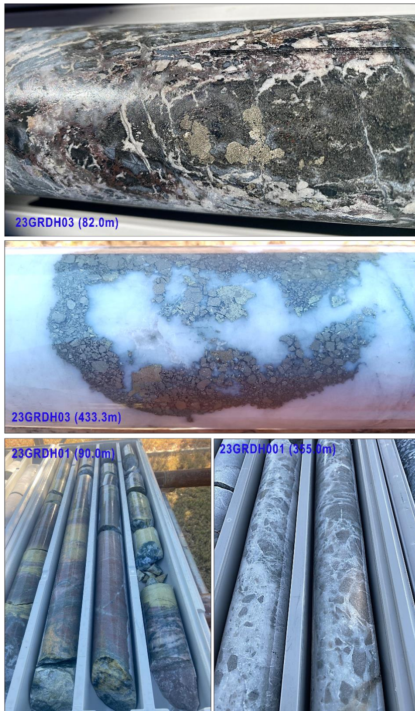
Figure 1: 23GRDH03 (82m): brecciation and sulphide infill of basalt; 23GRDH03 (433.3m): 400mm quartz-carbonate vein with early pyrite with later chalcopyrite; 23GRDH01 (90.0m): Strong epidote-silica-hematite alteration; 23GRDH001 (355.0m): large zones of brecciated quartz-dolomite veins with trace sulphide (pyrite).
