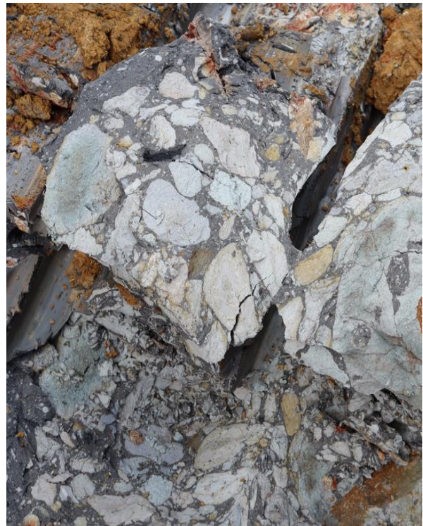
Generally, highly weathered with strong pervasive argillic alteration, characterised by strong pervasive hematite-limonite-clays. No primary sulphides are noted due to weathering.
