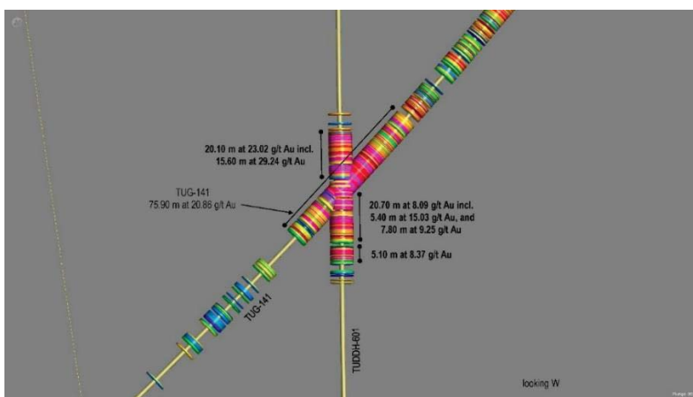
Figure 2: Vertical section looking West of the mineralized intervals in TUG-141 and TUDDH-601 that were drilled in essentially the same plane. Grades in ppm Au shown as colored discs are as follows: 0.1-0.2, blue; 0.2-0.3, light blue; 0.3-0.5, green; 0.5-1.0, yellow; 1-3, orange; 3-10, red; >10, fuschia.
