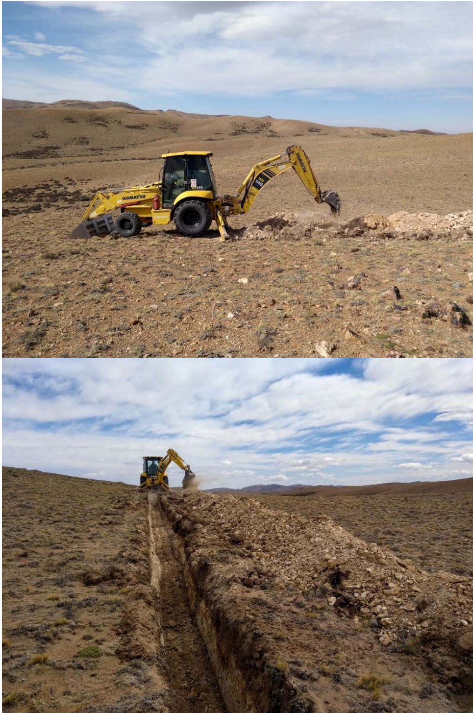
Image 1 – Trenching at Cachi Gold Project which has exposed the extension of known surface vein systems under soil and ash cover.
