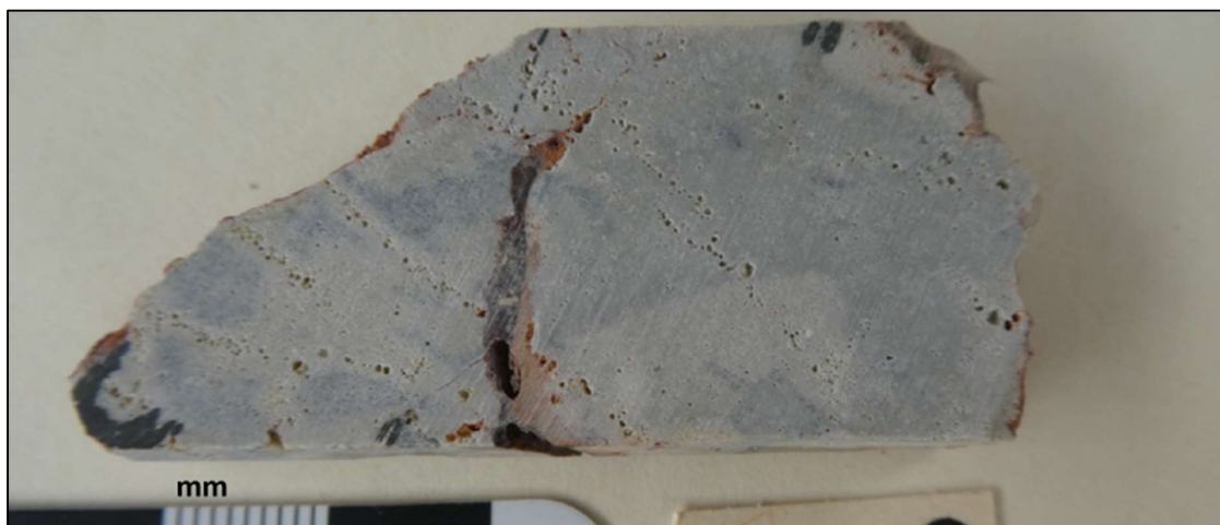
Photo 2 – Slab from Atlantis outcrop of sample KB03118 which returned 0.84g/t Gold 5 , dominated by secondary silica (hydrothermal alteration), containing abundant ex-sulphide coarse voids (up to 1mm) which are flanked by fibrous pressure fringe quartz.
