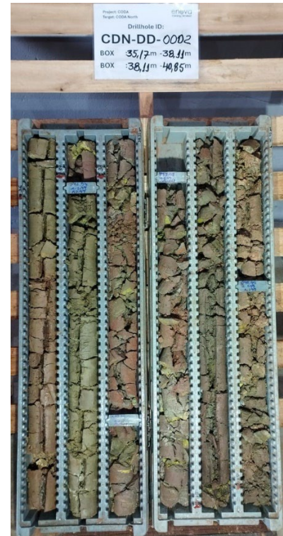
Figure 4: CDN-DD-0002 drill core which has been reported as having 14 m intercept @19.2% \text{TiO}_2
