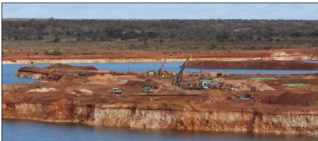
Figure 1: RC and diamond drilling at the Racetrack Prospect
