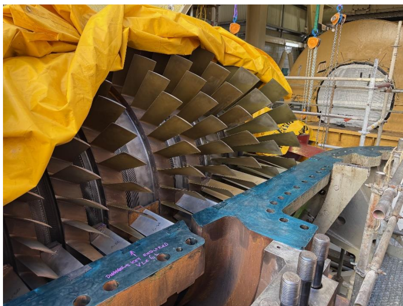
Image: Overhaul compressor stages of TPS turbine
