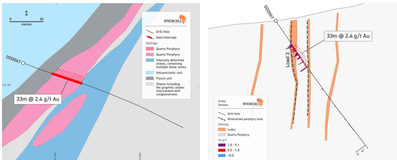
Figure 4: Details of the drillhole DDD047: (left) geological map of the DDD047 drillhole area, modified after Equigold 2010 prospecting data; (right) Cross section of prospect drawn through the drill hole DDD047.
