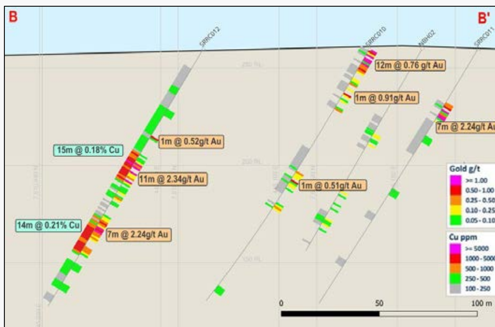
Figure 5-15: Cross section B–B' showing shallow gold anomalism intersected in drill holes SRRC011 and SRRC012
