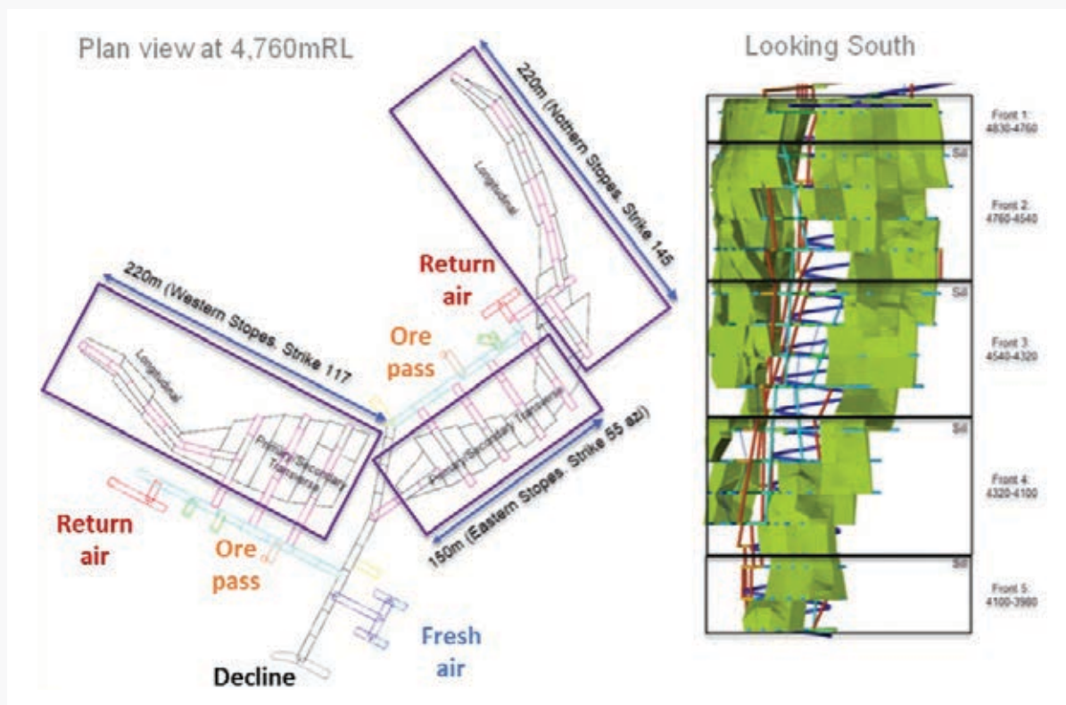
Figure 55: Typical SLOS mining level layout at Havieron
