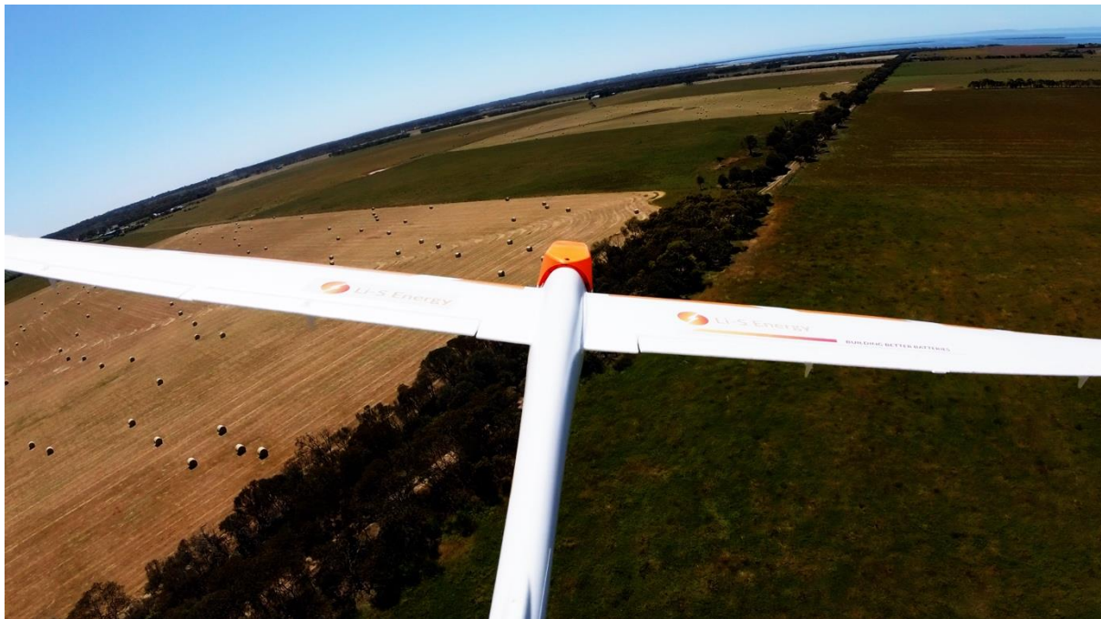
Uncrewed aircraft powered by an Li-S Energy lithium sulfur battery pack flies high over farmland in Southern Victoria during flight testing
