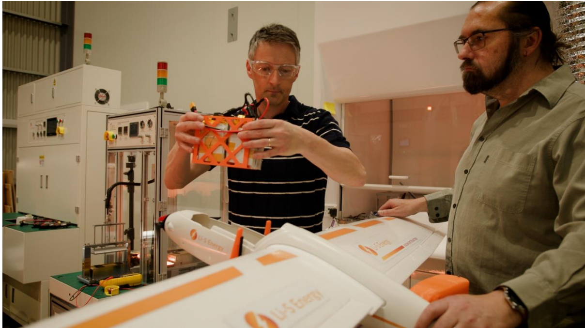
Li-S Energy battery pack being installed into the airframe before flight testing
