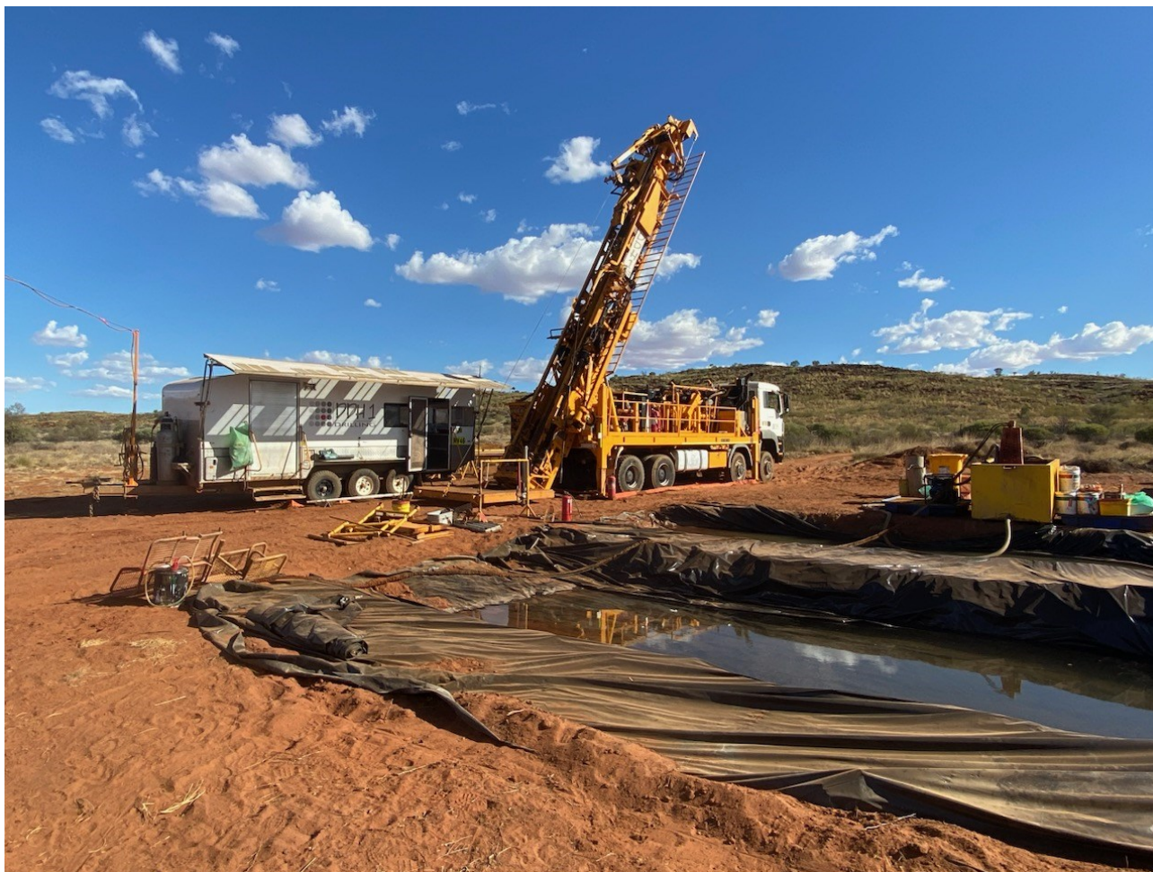
Image: Diamond drill rig set-up and ready to start the first hole, WADD001, at Pokali North.
