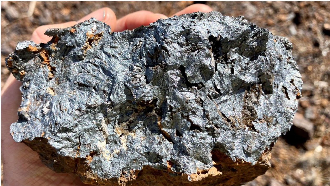
Figure 9. Manganite sample showing pyrolusite needles (Sample#ZEU110).
