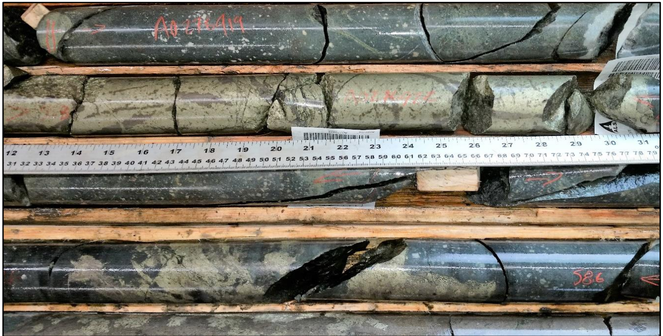
Figure 4: Core from the 4.1m zone of mineralisation hosted in Feldspar Porphyry assaying 5.3% Cu, 4.9g/t Pd, 0.9g/t Pt, 0.26% Ni, 12g/t Ag from 55.3m in ZA-19-05 (including the high-grade zone shown in Figure 2).
