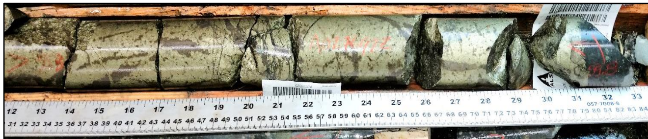
Figure 2: Hole ZA-19-05, 0.5m intersection of chalcopyrite - pyrrhotite massive sulphide from 55.3m hosted in feldspar porphyry assaying 22% Cu, 34g/t Pd, 3.5g/t Pt and 0.78% Ni, 1.4% Zn, 65g/t Ag.
