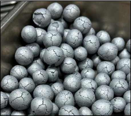
Metallised pellets after Linder test
