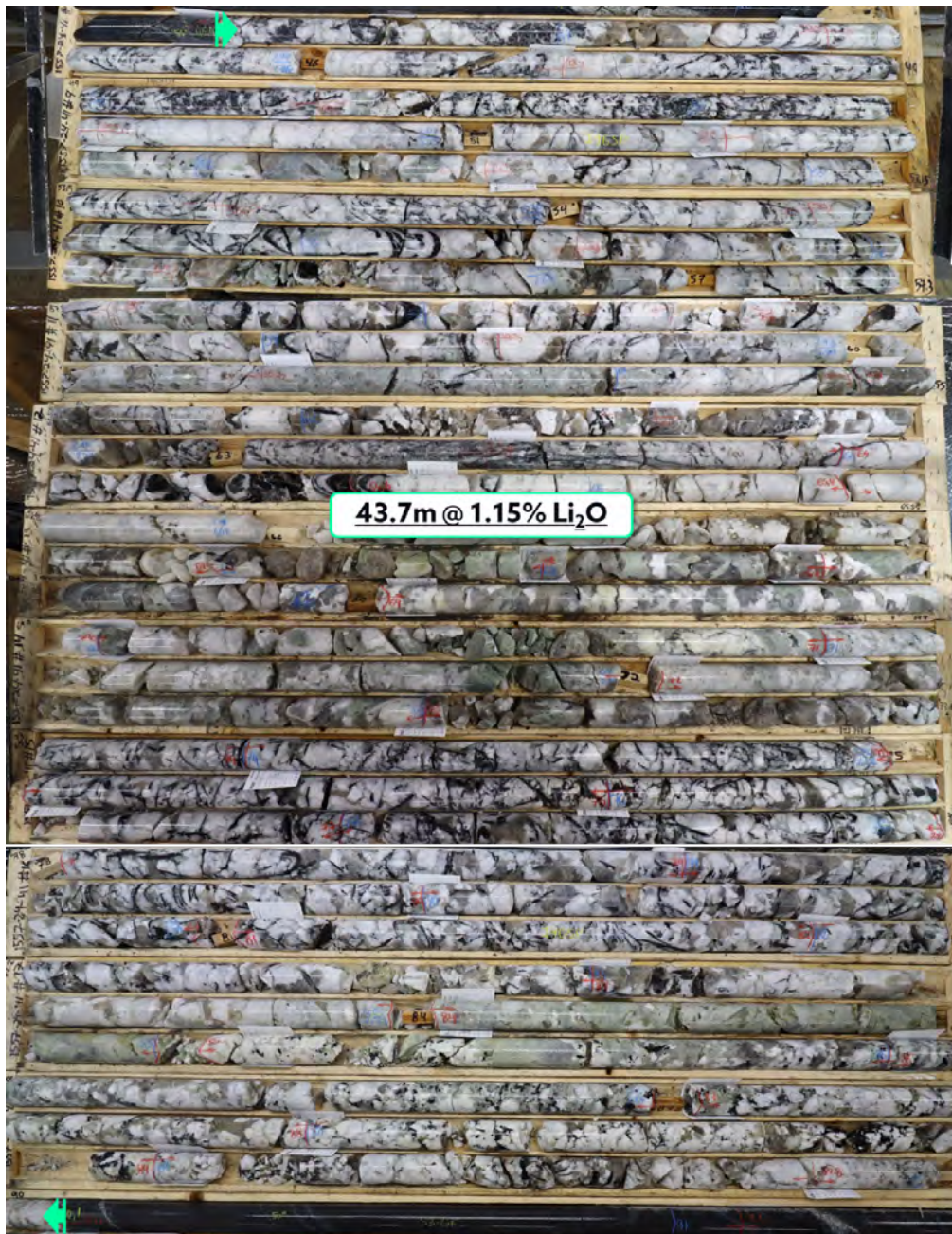
Figure 10: 43.7m at 1.15% \text{Li}_2\text{O} from 46.4m, including 4m at 3.0% \text{Li}_2\text{O} which includes 1m at 5.9% \text{Li}_2\text{O} in diamond drillhole 1557-24-041. 6
