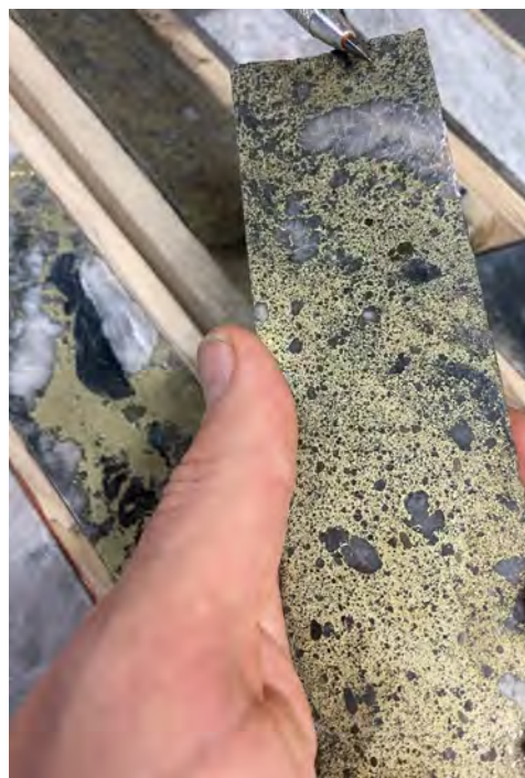
Figure 5: High grade drill core from CB-24-100 intersecting 7.3m at 4.2% Cu, 0.3g/t Au & 16.6g/t Ag. Image showing core between 321.9m and 322.6m. 5
