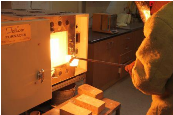
Removing deadburn magnesia from furnace
