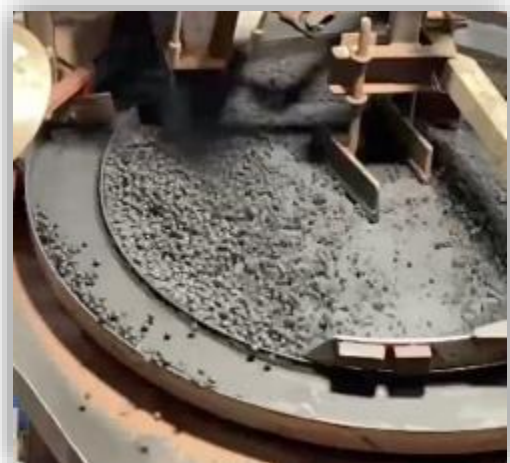
Picture 2. Green Ball manufacture in pelletising disc
