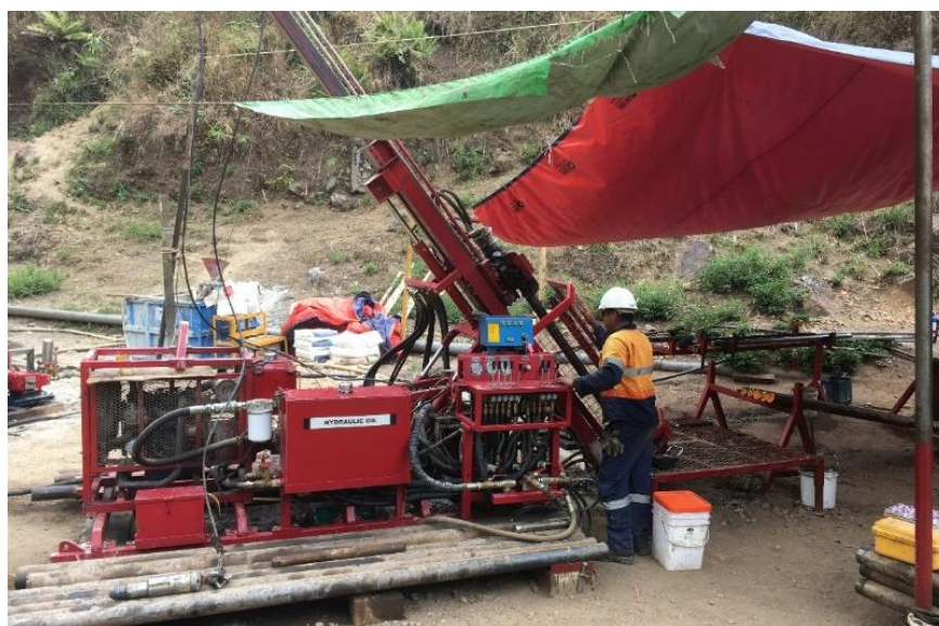
Figure 1. Shan North discovery hole BWDD030, being drilled by the man portable drill rig in the Bawdwin North village.
