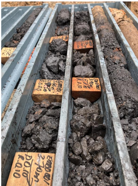
Figure 1: LEFT: EMDD001 core from 1.35 to 3.7m (Tray 1) RIGHT: Exploration Manager Steve Warriner at trench EMT01 Both the core and the trench contained 95% manganese oxides and 5% silicious manganese oxides
