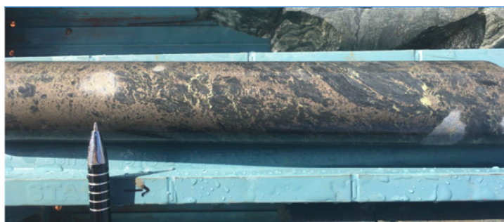
Figure 4 Wilga Downs Prospect - diamond core from hole 20WD001 at 552m depth showing semi-massive pyrrhotite (bronze colour) and chalcopyrite (yellow) \text{CuFeS}_2 mineralisation. Grade 1m @ 0.7% Cu and 0.7 g/t Au.
