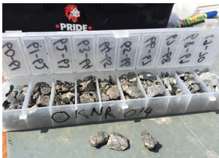
Figure 9: Massive sulphides in OKNR014 which returned 7m at 6.44% Zn and 0.43% Cu from 60m. Note each divider shows chips from a 1m interval.
