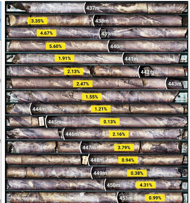
Diamond drill core from Severn hole ZS166 from approximately 436.5m – 451.4m. Core shows multi-stage pyrite-pyrrhotite-arsenopyrite vein network emplaced into strongly chloritized volcaniclastic sediments of the Crimson Creek Formation. Sn assays are shown in yellow as % Sn and depth intervals downhole in metres shown in white.
