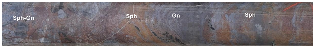
Massive Vein Mineralisation in NSD005 Core from 160.0m to 160.5m
