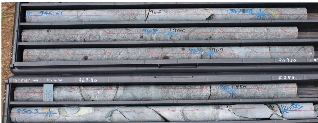
Photo One | Upper contact of the chilled margin of Unit A with the dunite of Unit B showing the fragments
