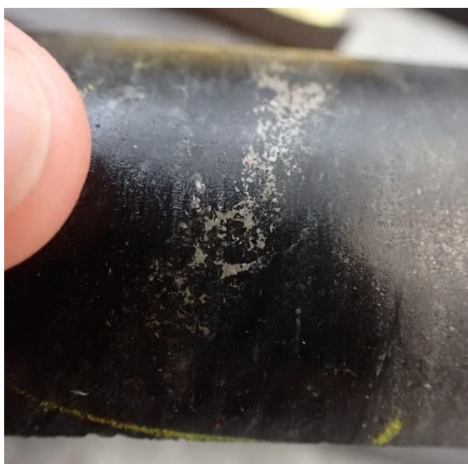
Photo Three | NQ2 core, 1,201.6m in hole PS414, pyrrhotite and chalcopyrite vein
