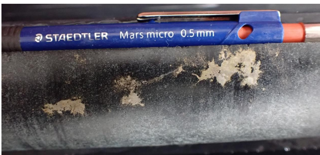
Photo Two | Pyrrhotite with Chalcopyrite blebs in Unit A at 1,095.3m in hole PS414
