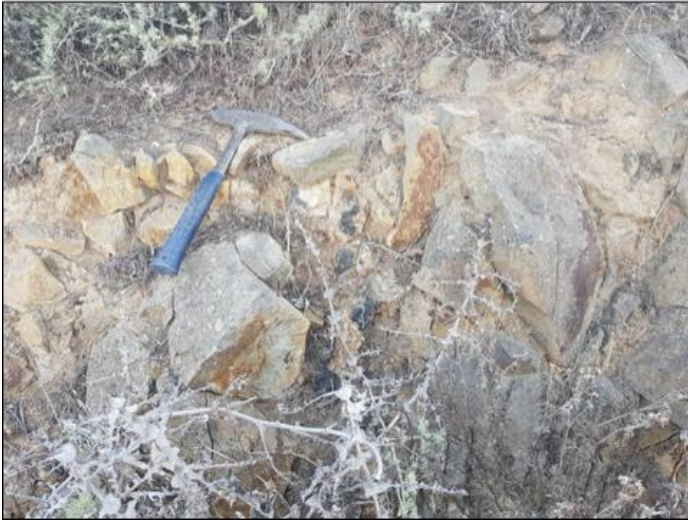
Image 2: El Dorado Magnetite sample grading +50% Fe
