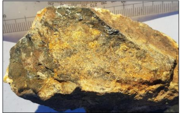
Image 2: El Dorado Magnetite sample grading +50% Fe
