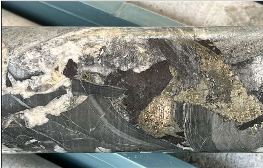
Figure 2. Photo of massive sulfides (predominantly pyrite and sphalerite (Zn-sulfide) in this section of core) infilling altered meta-sandstone breccia. (MPD002 - HQ3 diameter drill core).
