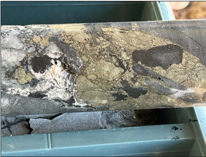
Figure 4. Fragments of massive sulfide in brecciated host rocks containing carbonate-quartz infill. Sulfides are predominantly pyrite and sphalerite. MPD002 approximately 210m down hole.
