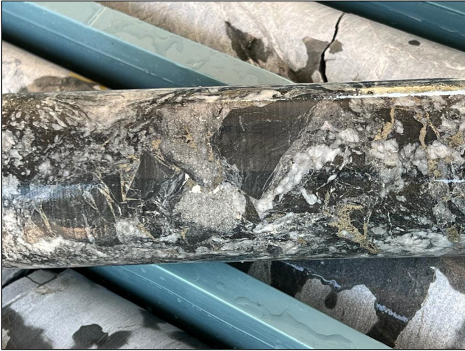
Figure 3. Photo of brecciated metasediments with quartz, carbonate, sulfide infill. MPD002 HQ3 diameter drill core.
