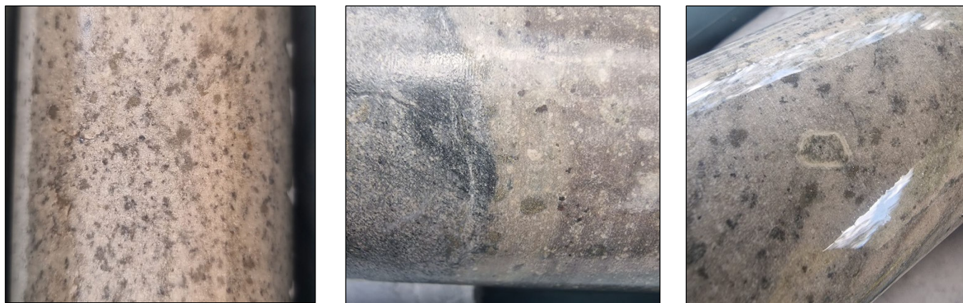
Figure 6. Examples of felsic intrusive (locally porphyritic) intersected at approximately 280m depth down hole. The intrusive rock shows varying degrees of alteration with pyrite replacing or partly primary grains (left and centre) and phenocrysts (right). Drill core is all HQ3 or part thereof. The photographs are from sections between approximately 280-290m down hole.
