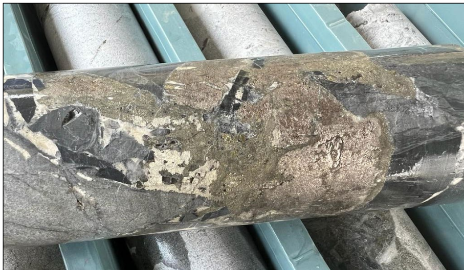
Figure 1. NMR are continuing to drill some impressive breccias at its Maneater Breccia Pipe in north Queensland. Breccia containing massive sulfide infilling breccia fragments. Sulfide mineralogy includes pyrite, chalcopyrite, sphalerite, +/- pyrrhotite. All core is HQ3 diameter. Depth of sample is 352m down hole. All drill core is HQ3.
