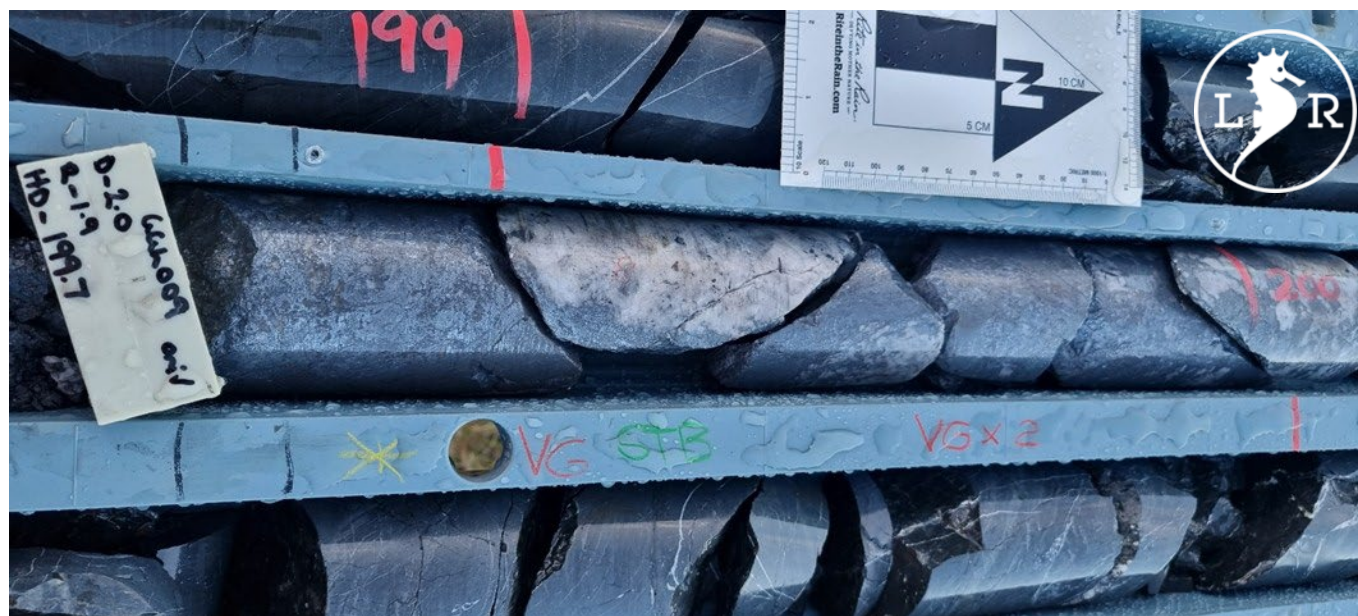
Figure 7 Drill core photograph from hole GGL009 (199.6m to 200.2m) showing massive stibnite and quartz veining containing visible gold (27.77 g/t Au and 27.17 % Sb)
