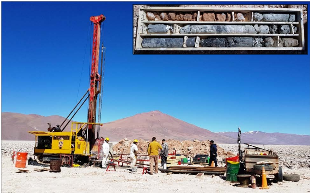
Photo 1. Rincon Lithium Project – Exploration diamond drilling operations and (inset) diamond drill core.
