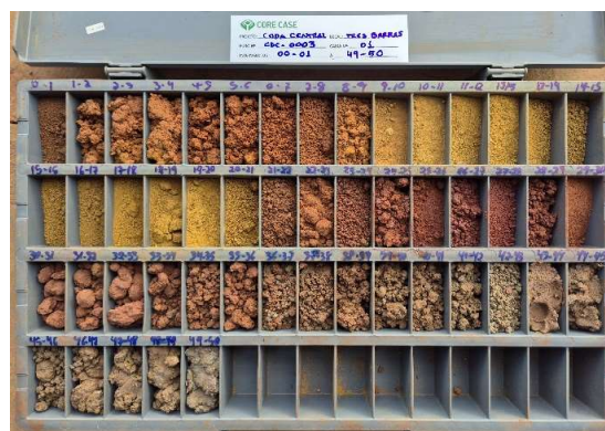
Figure 9: Variegated colour of drill cuttings from CDC-RC-003 hole, implying changes in lithology across undifferentiated sediment, laterite, kamafugite
