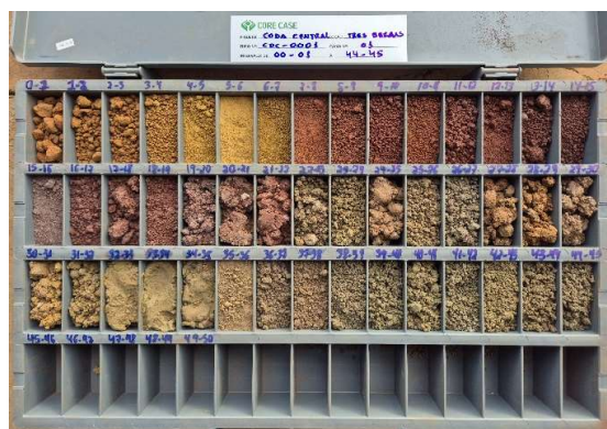
Figure 8: CDC-RC-001 drill hole cuttings of variegated colour of saprolite are stored in chip library
