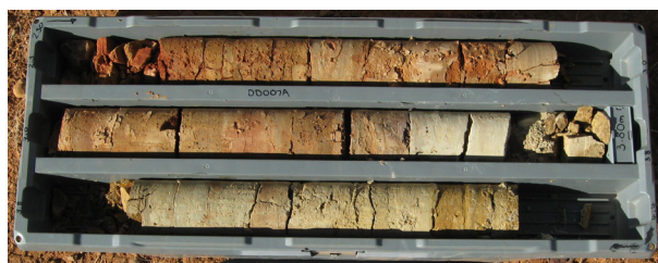
FIGURE: High-grade phosphate rock diamond drill core from mini-composite at Ardmore.
