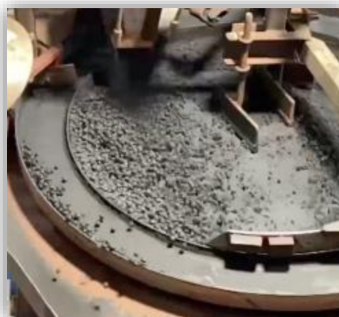
Picture 2. Green Ball manufacture in pelletising disc
