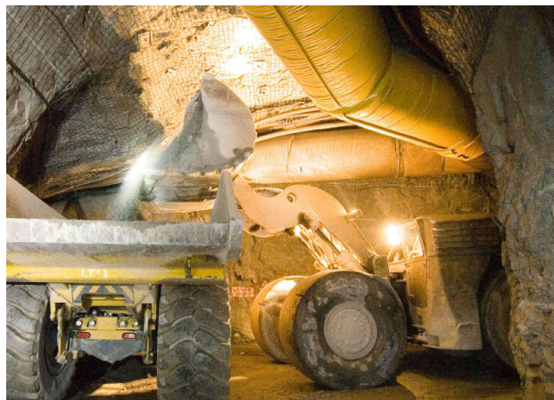
Underground during trial mining loading rock into truck for haulage to the surface. This was at the 'Warrior' mine, located about 5 kilometres from 'Central'. Future mining will be at 'Central' where there are many more reefs.
