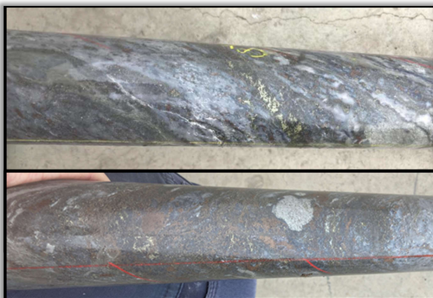
Figure 2: Massive zinc, lead and copper sulphide with quartz-sericite banding at approximately 225m downhole in HUD0030 – Assay Pending.
