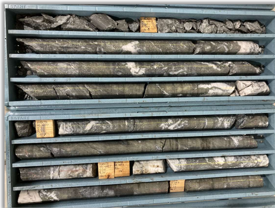
Figure 4 – Hume Target – Massive sulphides and quartz in HUD031 from 444.5m-451.0m within broader sulphide-rich interval from approximately 396m-451m – Assay Pending.
