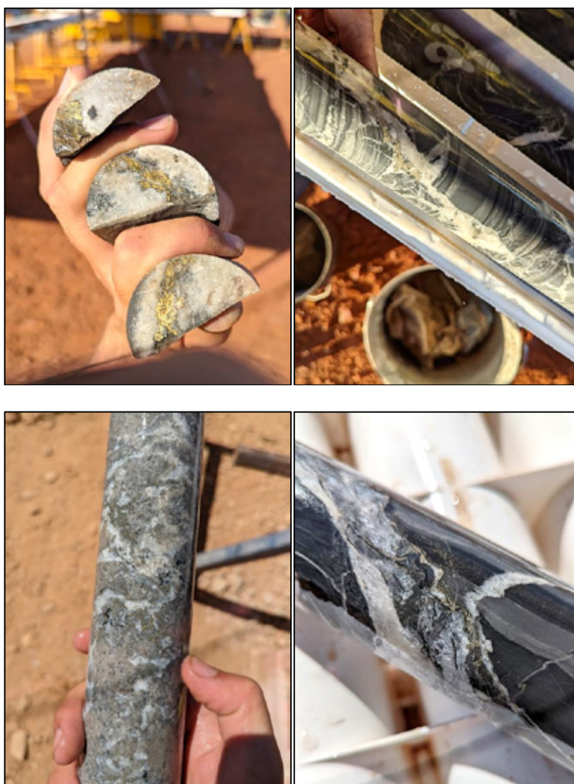
Photo's 1: Clockwise from top left – Chalcopyrite (cp) in quartz veining, pyrite (py) \pm cp along discordant quartz-carbonate veins selvage, py \pm cp veining with quartz-carbonate veining in siltstone, and fine disseminated pyrite in altered and brecciated Dolerite near apex zone.
