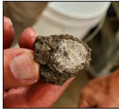
Figure 5: Fractured and partially wetted sample.
