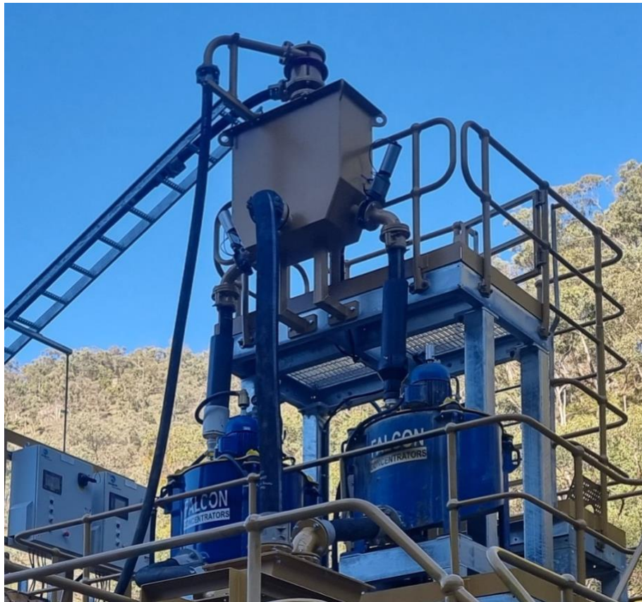
Figure 3 Reward gravity gold Falcon concentrators
