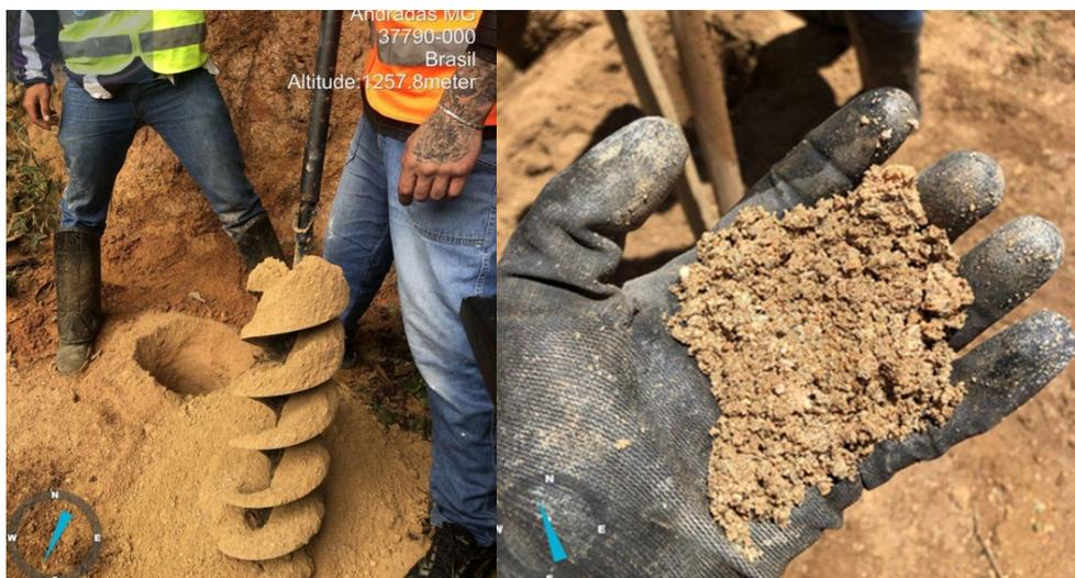
Figure 1: Manual auger drill sampling
