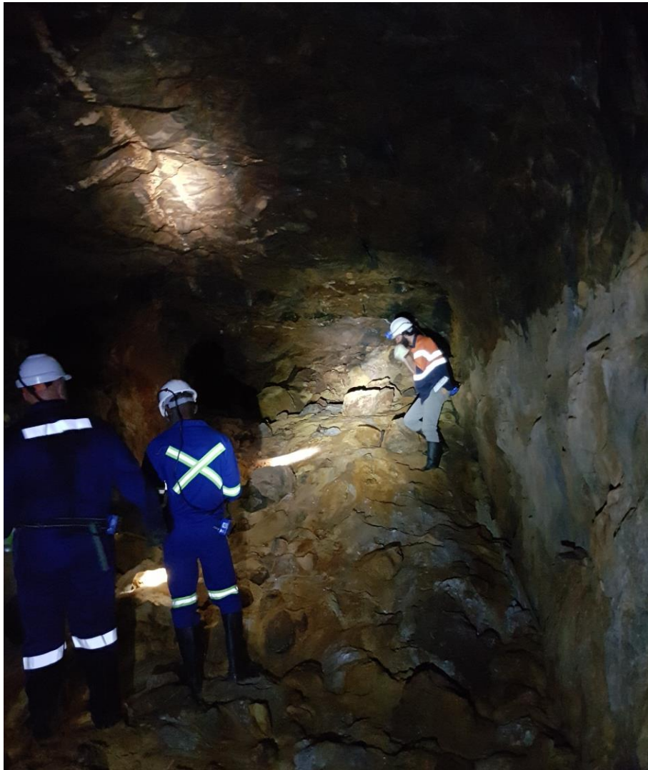
Figure 6: Orion's mining and geological team inspect blasted ore remaining in a draw point on 105 level. Note 1971 age paint marks remain on strong mine hanging-wall confirming no failure. Locality of picture is shown in Figure 5.
