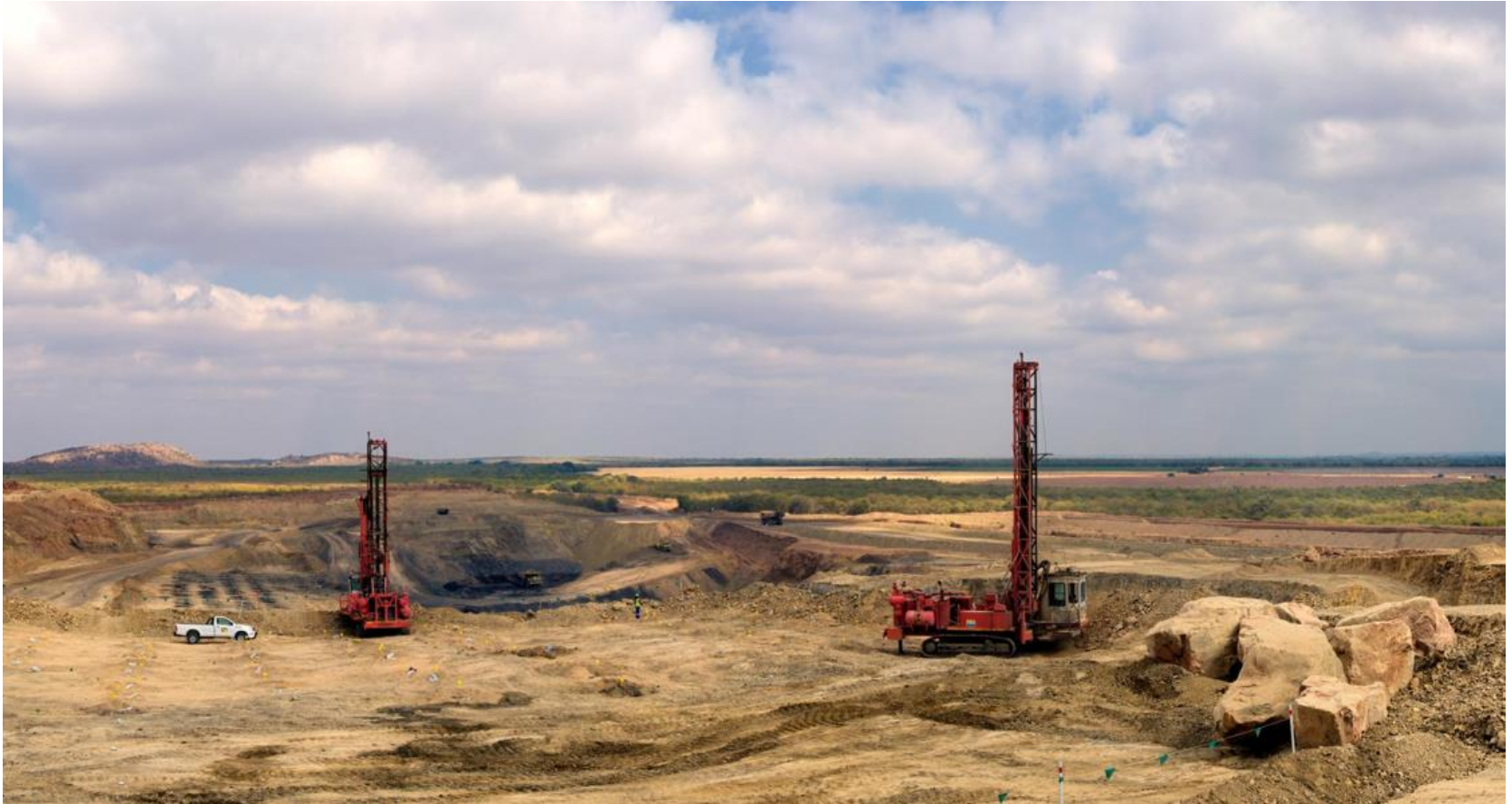
Blast drilling at the Vele Colliery
