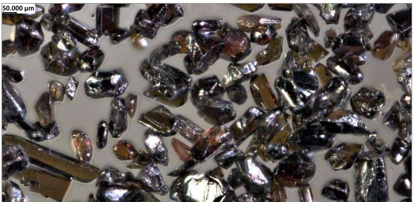
Figure 22: Photomicrograph of high purity rutile product 97.2% \text{TiO}_2
