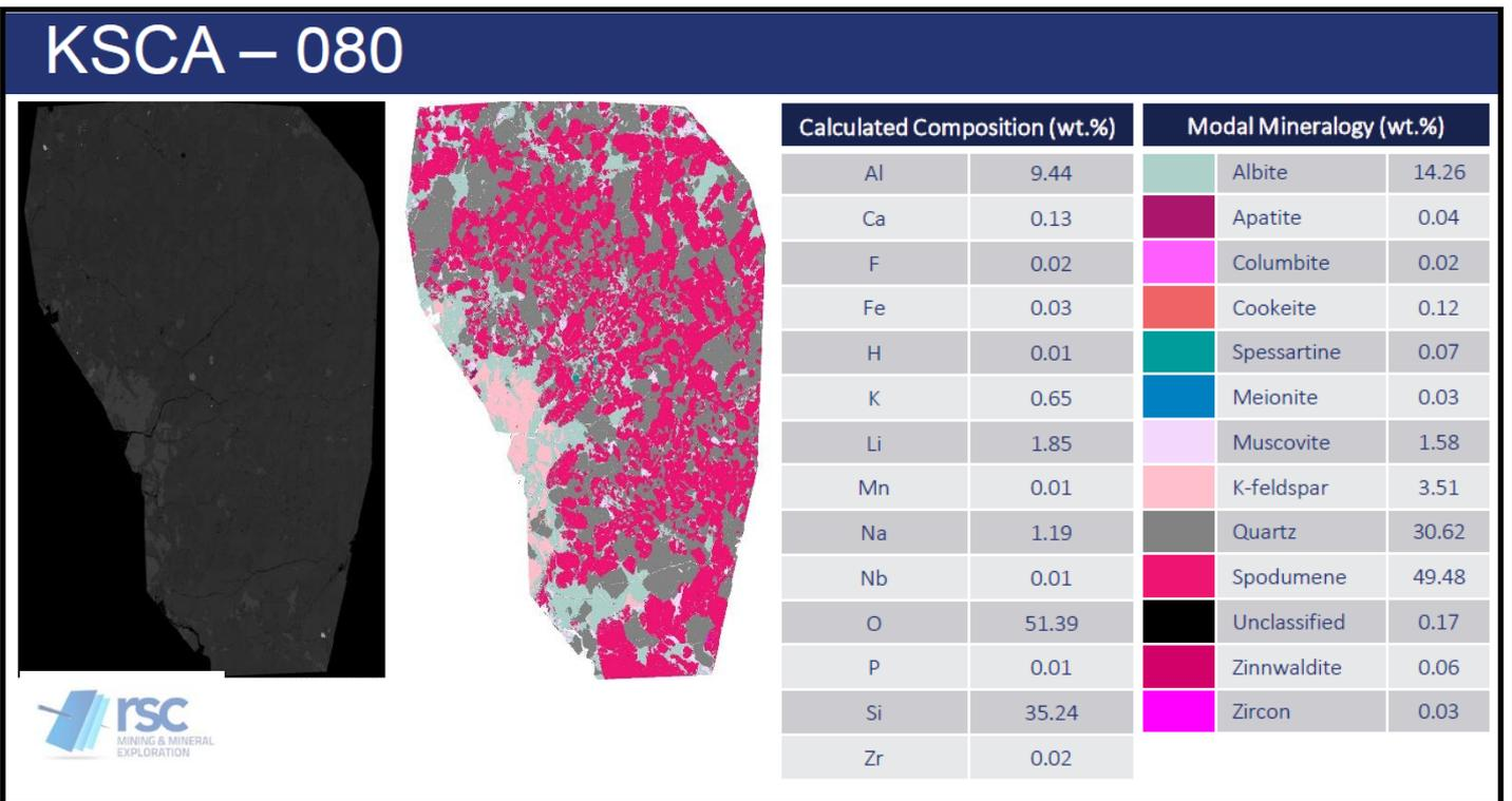
*Figure 3. SEM analysis of KSCA-080 showing calculated wt.% values*
