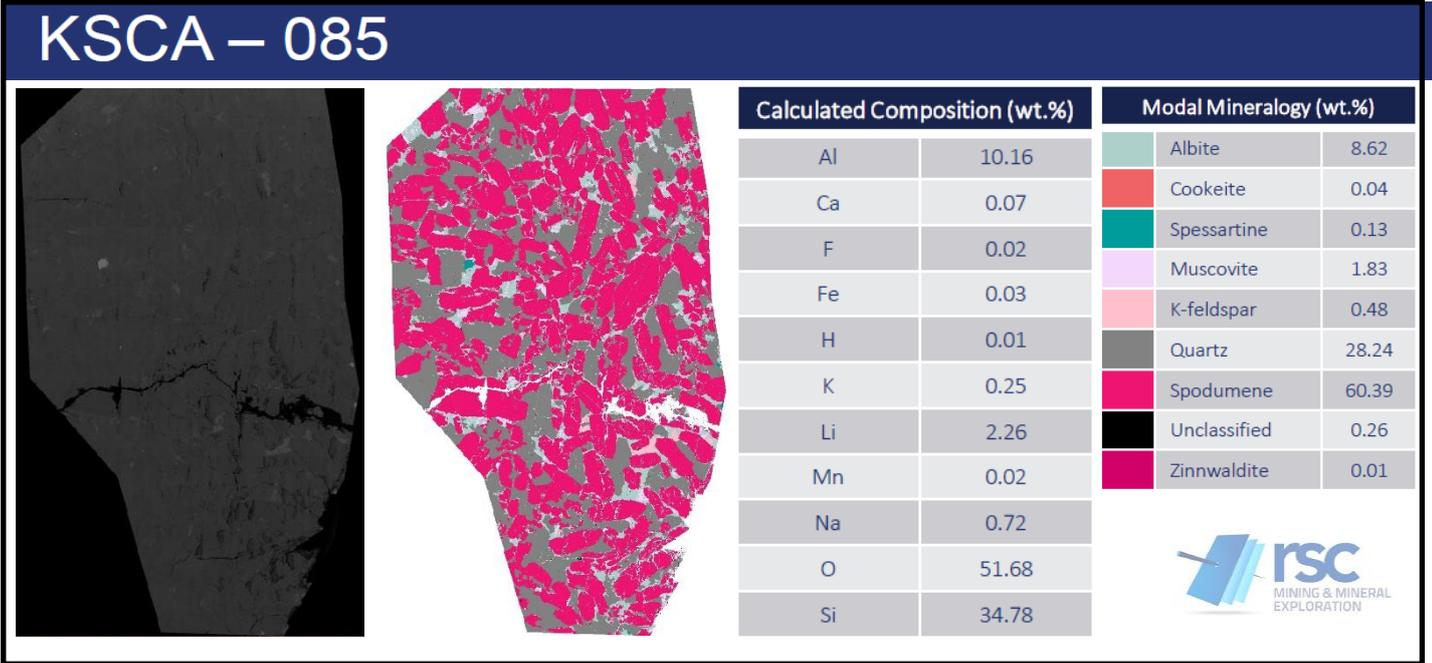
*Figure 2. SEM analysis of KSCA-085 showing calculated wt.% values*
