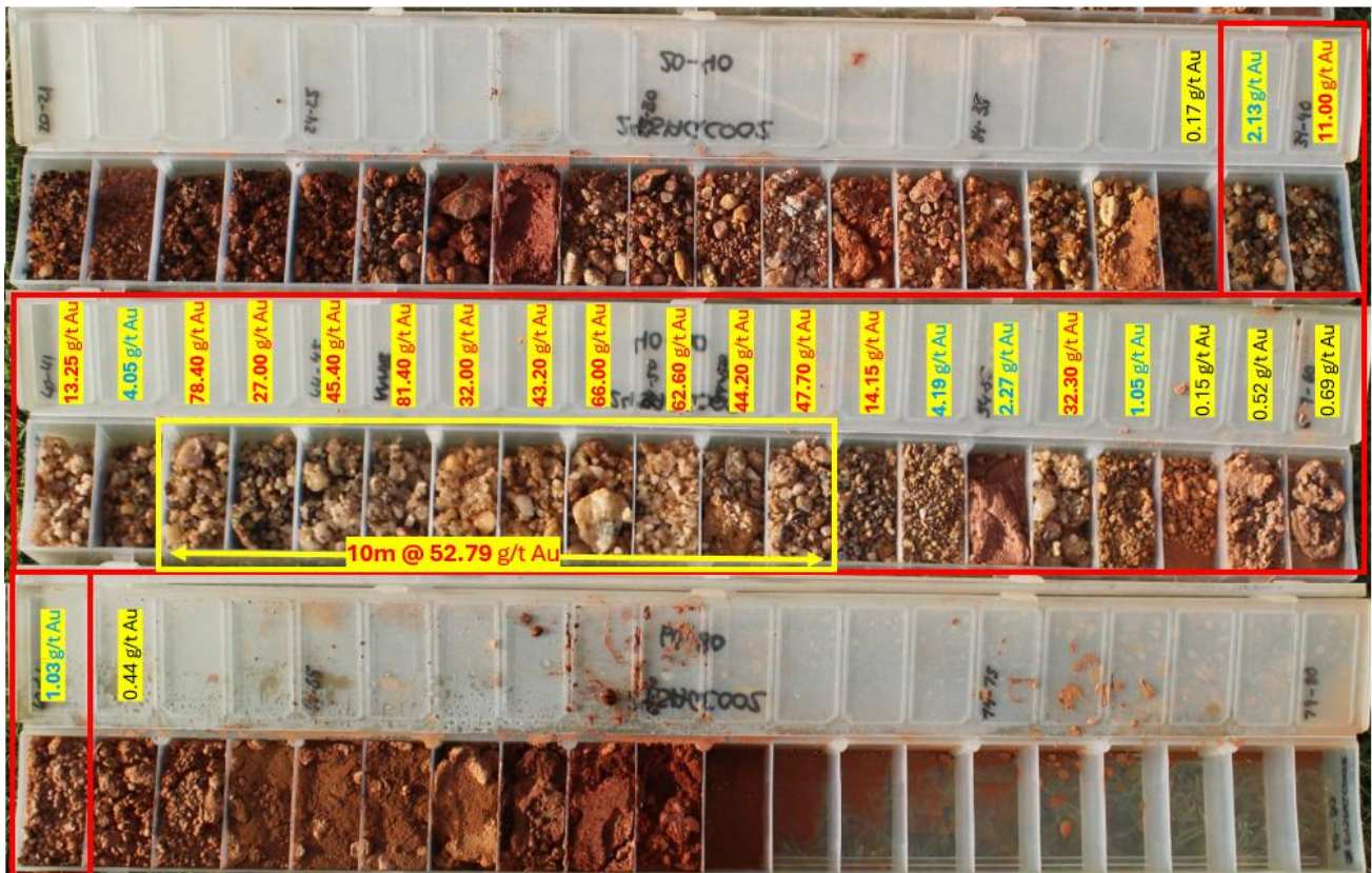
Figure 7: RC drill chips showing the quartz lode and bonanza gold zone, 23m @ 26.73g/t Au including 10m @ 52.79g/t Au , intersected in hole 24SAGC002.
