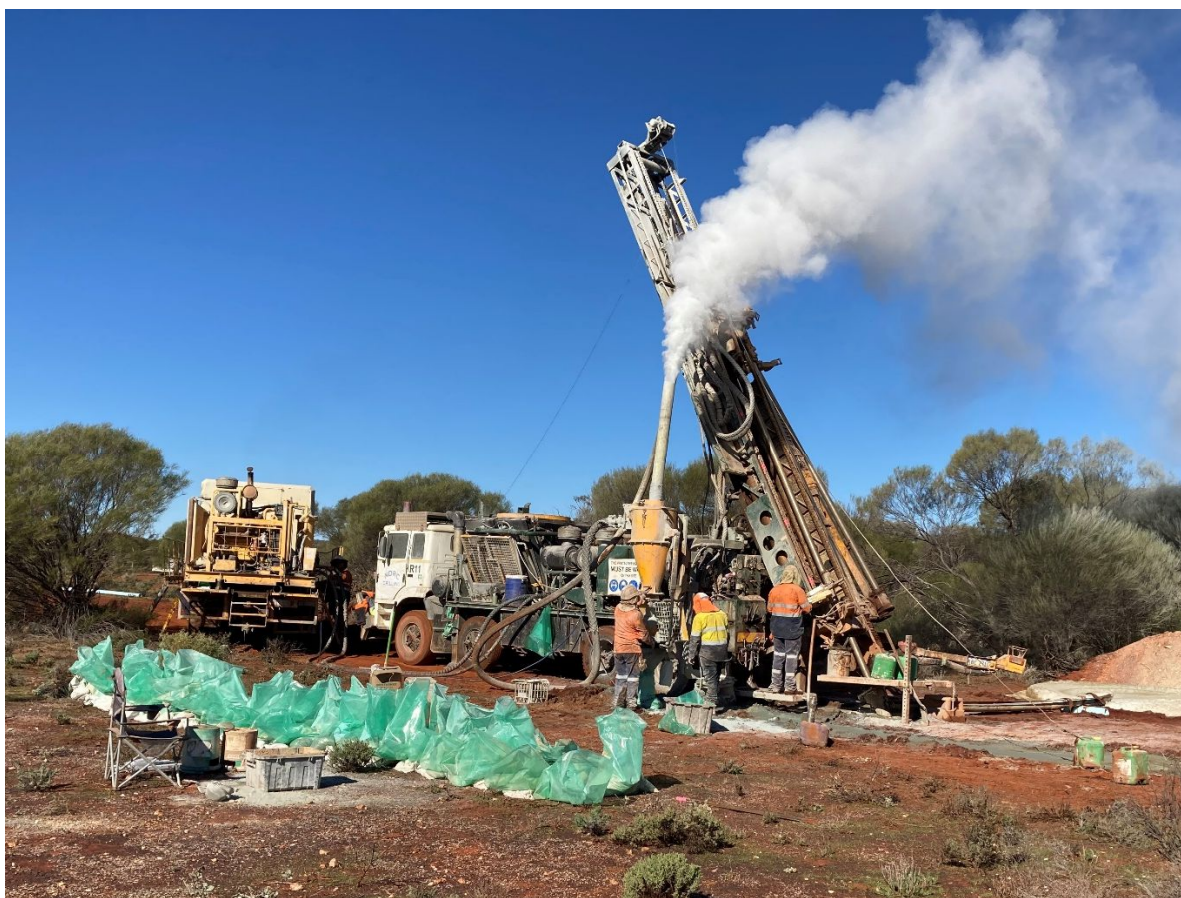
Plate 2: Reverse Circulation drill rig on site at Yidby Gold main zone.
