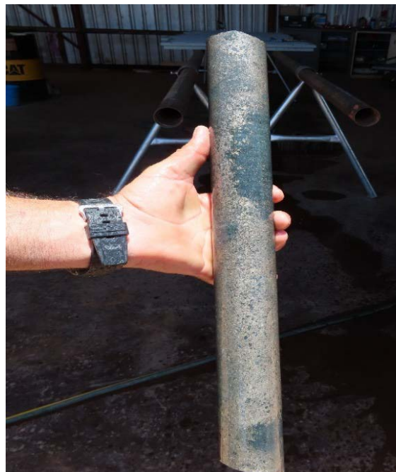
Photo 2: ANDD0012 drill core Semi-massive Ni-Cu sulphides @ 84.1-85.0m downhole
