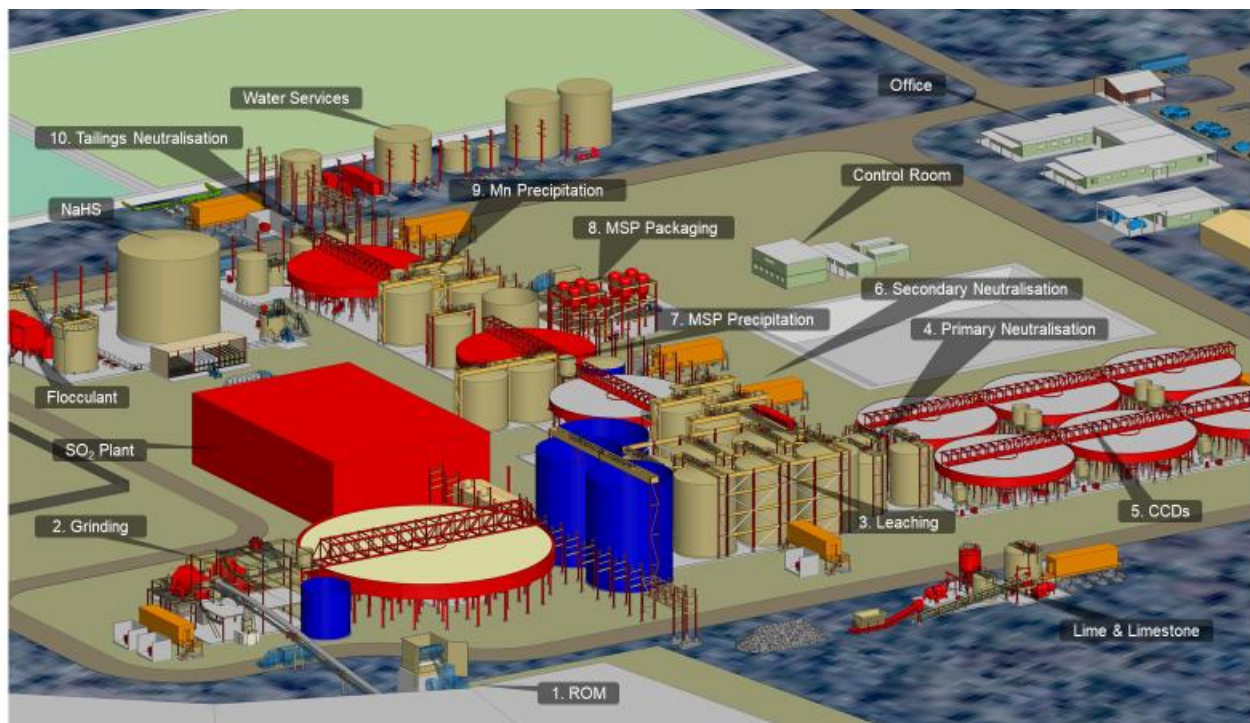
Figure 4 – 3D isometric of the Mt Thirsty processing plant showing generalised process flow (numbered labels)
